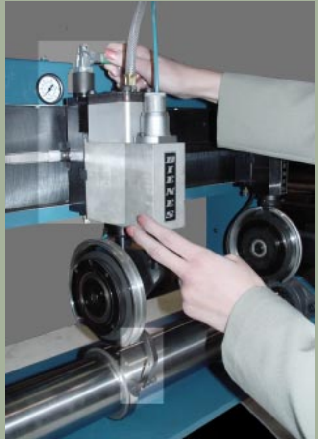
Highlighted are the CLB system and the ES Tab ® locating tool for quick and reliable manual knife set up.
