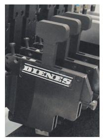
**The PQAS 1/2 Mechanical Holder** allows blade replacement without holder removal. Individual blade holder slides can be preloaded with fresh blades for common, quick, and safe exchange when needed. A quick pin locking system allows placing the blade out of harm's way during thread up.
