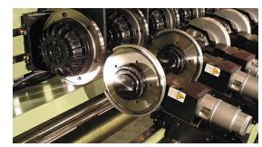
**SHAFT DRIVEN** QUICK SET systems bottom knives mount to precision traversing carriages that prevent excessive axial run-out and shaft deflection. This capability allows for unlimited shaft lengths,
