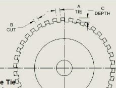
Note: The depth of the Ties is what we would like to have. However, if this is not possible, please indicate the depth which can be machined.
